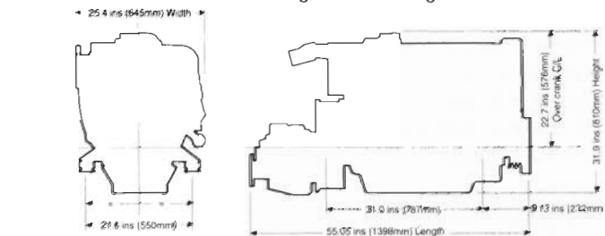
Perkins Sabre M130C with Newage PRM 500D gearbox
